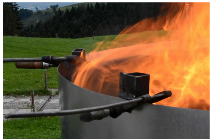
Fig. 8: Air is drawn in over the hot outer wall of the kiln and swirls above the fuel bed creating a vortex that ensures good mixing of pyrolysis and combustion air, resulting in very low emissions of the Kon-Tiki kiln.
